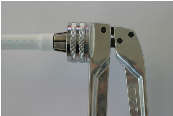
Figure 1. Showing the correct method for using the widening tool for expanding the pipe prior to insertion of the pipe into the fitting – expand once.
