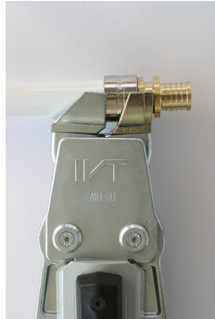
Figure 2. Showing the correct method for using the gripper tool for placing the sleeve over the pipe after insertion of the pipe onto the fitting.
