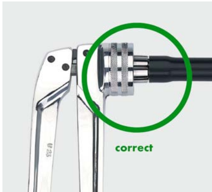
Figure 1. Showing the correct method for using the widening tool for expanding the pipe prior to insertion of the pipe into the fitting. The pipe end should be expanded twice.
